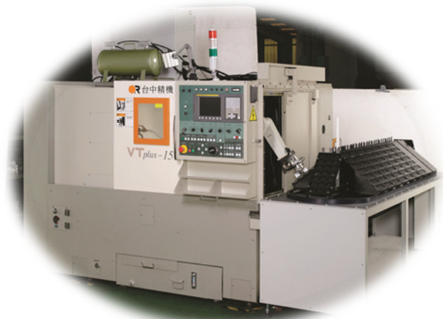
Single lathe with articulated robot
