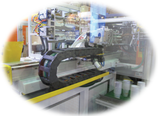
Mold injection with robot for auto part unloading.
