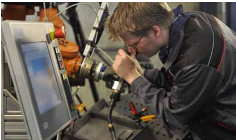
Teaching an industrial robot by demonstration
