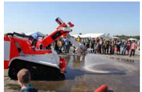
HARDY - Multipurpose service, emergency and rescue tracked robot (cooperation with Strojírny Třinec a.s., Fite a.s. Ostrava, Robotssystem s.r.o.).
