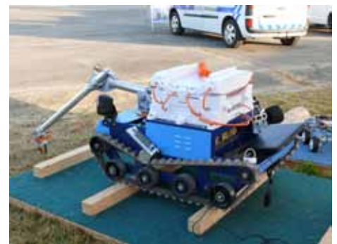
ARES – mobile robot for collection of liquid, gas and solid samples, exploration and manipulation.
